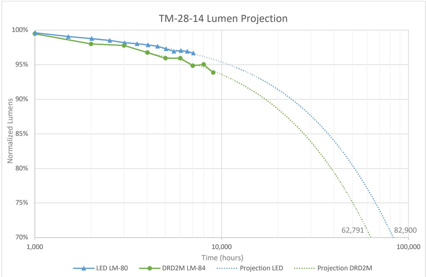
The LED data is also included from the LED manufacturers published LM-80 file<sup>6</sup>. Notice how the LED extrapolation indicates better lumen maintenance over time than the modules, illustrating that using only LED LM-80 based information extrapolations can provide an optimistic prediction of longevity.
